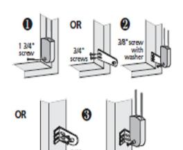
recess the shade, the flat surface must be at least 2° deep. Add to these minimum depths the dimension of any obstruction to shade movement, such as a window crank or handle. Two screws are used to attach each bracket. Mount the brackets at the locations you marked, with their front edges aligned.
